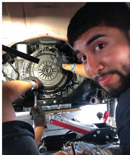
Sal and Tito install a new clutch
