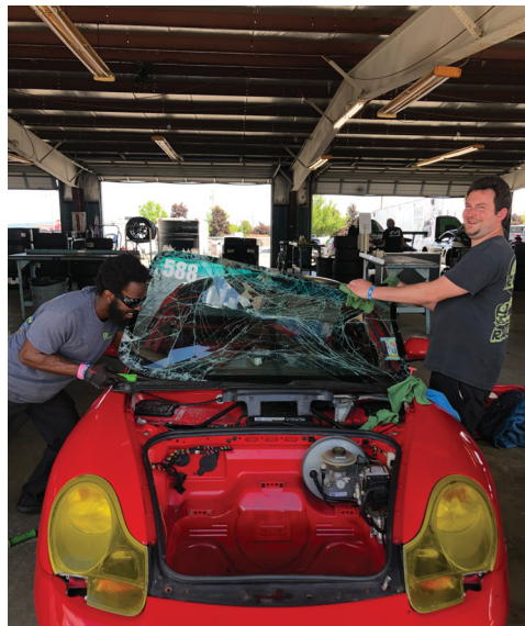
Brian and Otis remove the broken windshield
